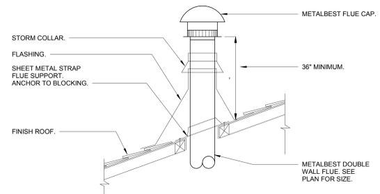
**J FLUE THRU ROOF DETAIL**
