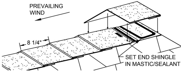
FOR THE LAST SHINGLE OF THE RUN, REMOVE THE CUTOUT END OF THE RIDGE SHINGLE AND TRIM TO FIT, MAINTAINING THE 8 1/4" EXPOSURE. SET THE SHINGLE IN MASTIC.
