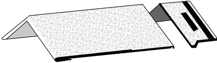
TO CREATE AN EZ-RIDGE STARTER, CUT OFF THE 8 1/4" EXPOSURE PORTION\* OF AN EZ-RIDGE SHINGLE, AND USE THE 3 1/4" REMAINDER (WITH SEAL-DOWN STRIP) AS THE STARTER.
