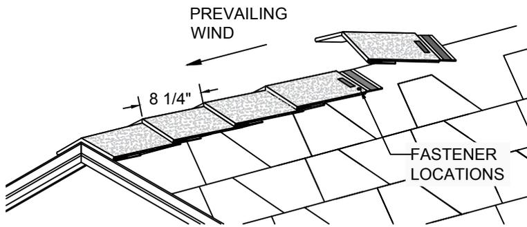
FIRST EZ-RIDGE SHINGLE COMPLETELY OVERLAPS STARTER. POSITION EACH EZ-RIDGE SHINGLE TO FOLLOW WITH AN 8 1/4" EXPOSURE BEFORE FASTENING.
