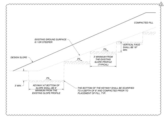
**D** FILL ON EXISTING SLOPE STEEPER THAN 6:1
