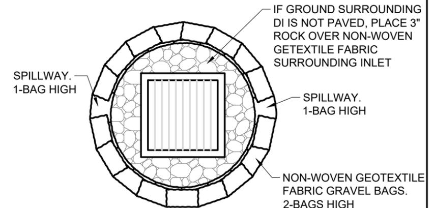
**SE 10a** LEVEL GRADE DRAIN INLET PROTECTION
