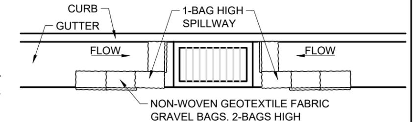
**SE 10b** CURB & GUTTER DRAIN INLET PROTECTION
