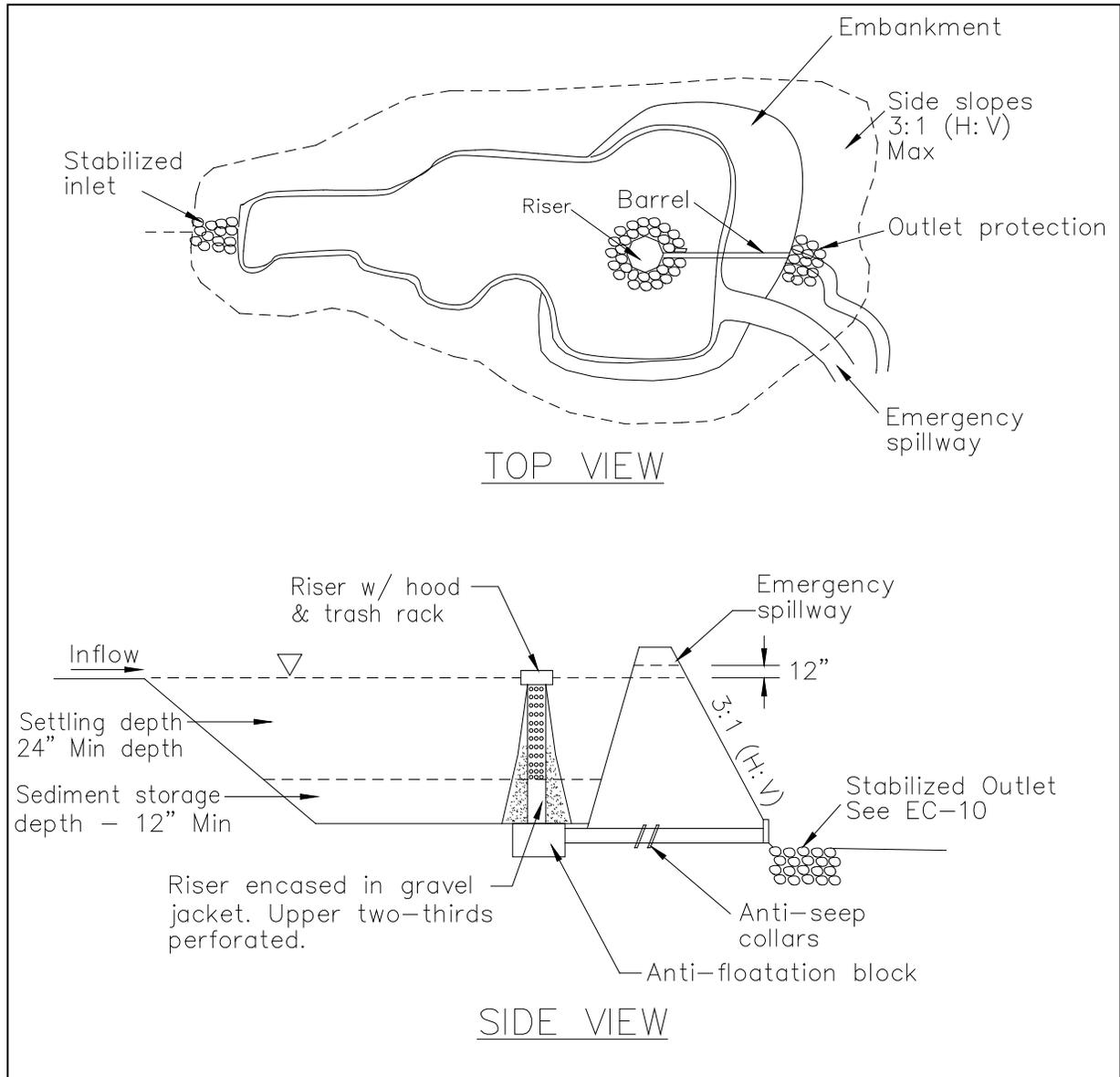
**FIGURE 1: TYPICAL TEMPORARY SEDIMENT BASIN
