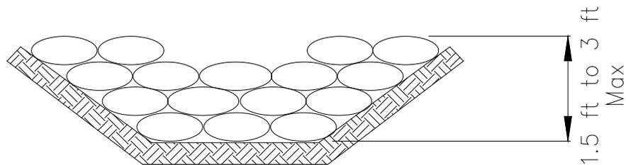
GRAVEL BAG CHECK DAM ELEVATION
