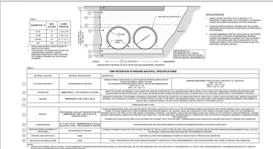
MANUFACTURER RECOMMENDED BACKFILL NOT TO SCALE
